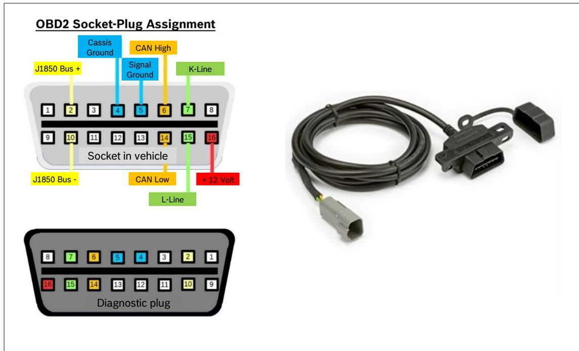
Figure 5: OBD2 socket with assignment and adapter cable
