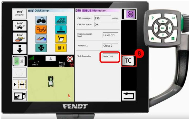
(8) If the TC is off, the “TC” button is not highlighted, and the status is inactive.
