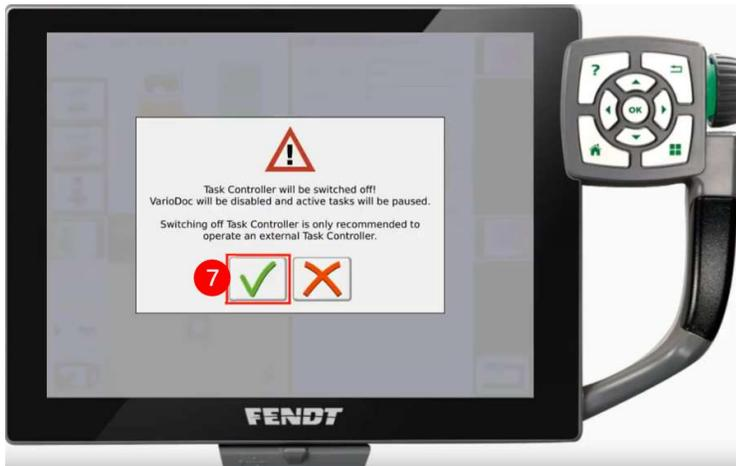
(7) Tab the “Check Mark” to confirm that the Task Controller shall be switched off
